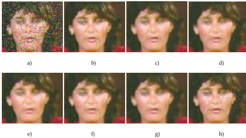
Fig. 4. a) Zoomed image region of 10th Miss America frame contaminated by impulsive noise of 15% intensity, b) Designed 3D-FCF , c) 3D-MF ; d) 3D-VVMF , e) 3D-VGVDF , f) 3D-VAVDATM ; g) 3D-VATM ; h) 3D-VKNNF .
